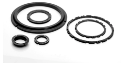
The rings that make the dynamic face seal are both lapped flat and are held together with springs or magnets so that liquids cannot flow between the ring faces even though they are spinning against each other at high rpm.
